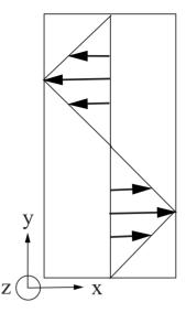
FIG. 1. Schematic diagrams of a zigzag velocity flow. The arrows represent the velocity vectors of the host fluid in the flow direction. The x, y, and z axes represent the flow, velocity-gradient, and vorticity directions, respectively.
