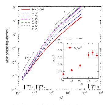
FIG. 3. (Color online) The time evolution of the mean-square displacement in the vorticity direction (z) for several volume fractions  $\Phi$  at  $k_BT$ =0.07 and  $\dot{\gamma}$ =0.005. The Peclet number Pe  $\approx$  170 and the particle Reynolds number Re<sub>p</sub>=0.125. The inset shows the volume fraction dependence of  $D_z$  scaled by  $\dot{\gamma}a^2$ . The parameters for both the particle and fluid are a=5,  $\xi$ =2,  $\rho_p$ =1,  $\rho_f$ =1, and  $\eta$ =1.
