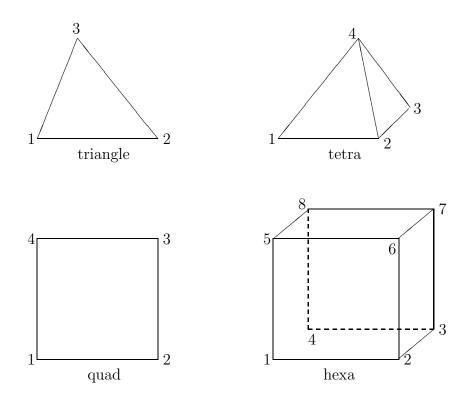
Figure 3.1: Node order of a contour element
