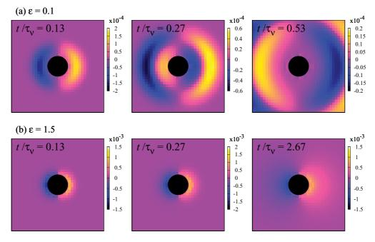
FIG. 2. (Color online) Time evolution of the fluid density deviation around the particle. The compressibility factors are (a)  $\varepsilon = 0.1$  and (b)  $\varepsilon = 1.5$ . The color scale (gray scale) represents negative (darker) to positive (lighter) density deviation. The black circle represents the particle. The direction of the initial particle velocity is right in these pictures.
