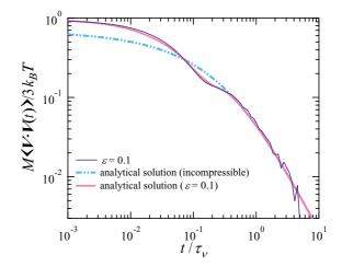
FIG. 5. (Color online) The velocity autocorrelation function at  $\varepsilon = 0.1$  and  $k_B T = 10^{-4}$ . The bold solid line represents the analytic solution of the velocity relaxation function. The bold dashed double-dotted line shows the analytic solution for an incompressible fluid.
