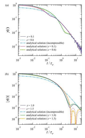
FIG. 1. (Color online) The velocity relaxation function for various compressibility factors: (a)  $\varepsilon = 0.1$ , 0.6, (b) 1.0, and 1.5. The bold lines illustrate the analytic solutions for various compressibility factors, and the bold dashed double-dotted line shows the analytic solution for an incompressible fluid.
