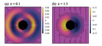
FIG. 4. (Color online) The fluid velocity field and its divergence,  $\nabla \cdot \mathbf{v}$ , at  $t/\tau_{\nu} = 0.27$ . The values are normalized by the factor  $Ma^*/|\mathbf{P}|$ . The compressibility factors are (a)  $\varepsilon = 0.1$  and (b)  $\varepsilon = 1.5$ . The color scale (gray scale) represents negative (darker) to positive (lighter) divergence. The black circle represents the particle. The direction of the initial particle velocity is right in these pictures.
