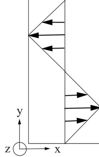
FIG. 1. Schematic diagrams of a zigzag velocity flow. The arrows represent the velocity vectors of the host fluid in the flow direction. The  $x$ ,  $y$ , and  $z$  axes represent the flow, velocity-gradient, and vorticity directions, respectively.
