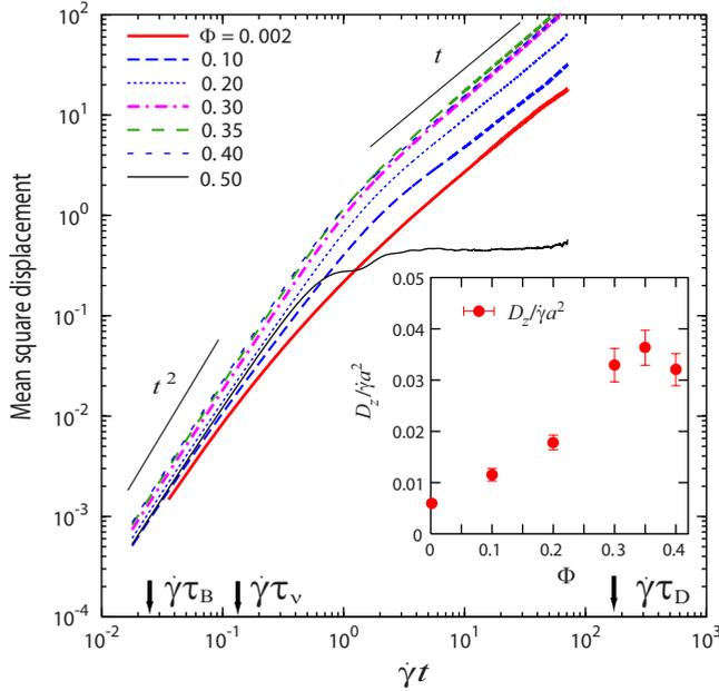
FIG. 3. (Color online) The time evolution of the mean-square displacement in the vorticity direction ( $z$ ) for several volume fractions  $\Phi$  at  $k_B T = 0.07$  and  $\dot{\gamma} = 0.005$ . The Peclet number  $Pe = 170$  and the particle Reynolds number  $Re_p = 0.125$ . The inset shows the volume fraction dependence of  $D_z$  scaled by  $\dot{\gamma}a^2$ . The parameters for both the particle and fluid are  $a = 5$ ,  $\xi = 2$ ,  $\rho_p = 1$ ,  $\rho_f = 1$ , and  $\eta = 1$ .
